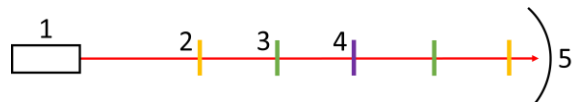
Fig. 9: Schematic experimental setup for the Hadamard and Z gate demonstration: 1. laser, 2. horizontal polarizer, 3. Hadamard gate, 4. Z gate, 5. detector
