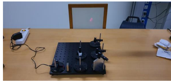
Fig. 3: C-NOT experiment realizing the input qubit states through the usage of a vertical polarizer and the rotation of the laser, creating an antidiagonal oval.
