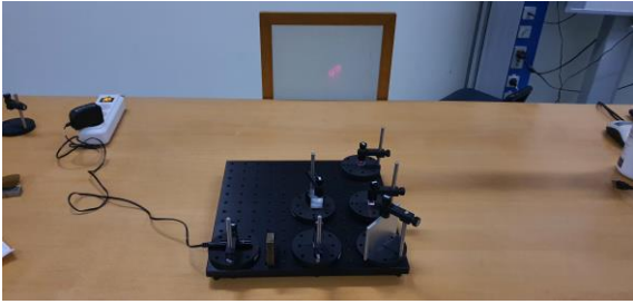
Fig. 6: C-NOT experiment realizing the input qubit states through the usage of a horizontal polarizer and the rotation of the laser, creating a diagonal oval.
