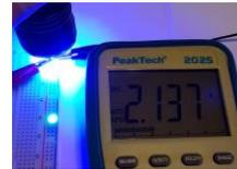
Fig. 3: A LED is illuminated and provides the voltage  $U = 2.137$  V and electrons with the energy  $E = 2.137$  eV.
