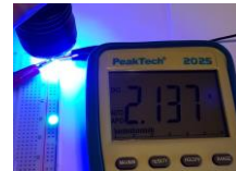
Fig. 3: A LED is illuminated and provides the voltage U = 2.137 V and electrons with the energy E = 2.137 eV.
