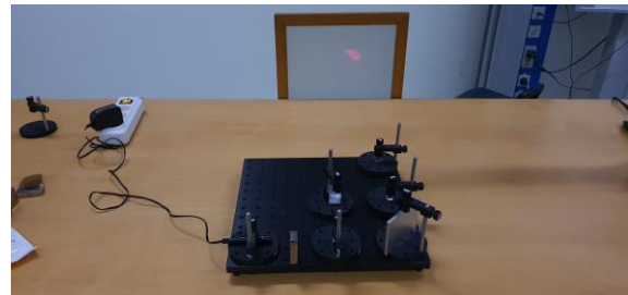
Fig. 4: C-NOT experiment realizing the input qubit states through the usage of a vertical polarizer and the rotation of the laser, creating a diagonal oval.
