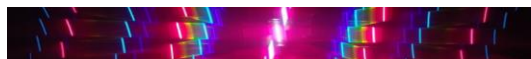
Fig. 2: Wavelengths of light can be measured. This photo of a hydrogen lamp is taken by a smartphone camera with a cross-grating in front of the lens.
