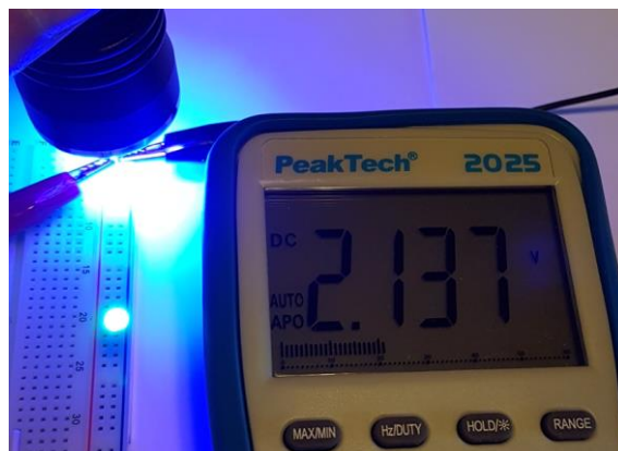
Fig.1: Students expose a blue LED to the light of a pocket lamp. The LED transforms the energy of the light into electric energy. With it, the connected green LED at pin 20 begins to shine. Moreover, the students attach two crocodile clips to the pins of the blue LED and to a Voltmeter. So they find out that the LED generates 2.137 V.
