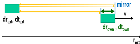
Fig.5: An observer moving at the box with two mirrors measures the light-travel distance dr_{own} between the mirrors. An external observer at rest in his system r_{ext} measures the light-travel distance dr_{ext} between the same mirrors.
