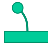
Fig.9: In this model experiment of an acceleration sensor, the sensor is accelerated to the right.
