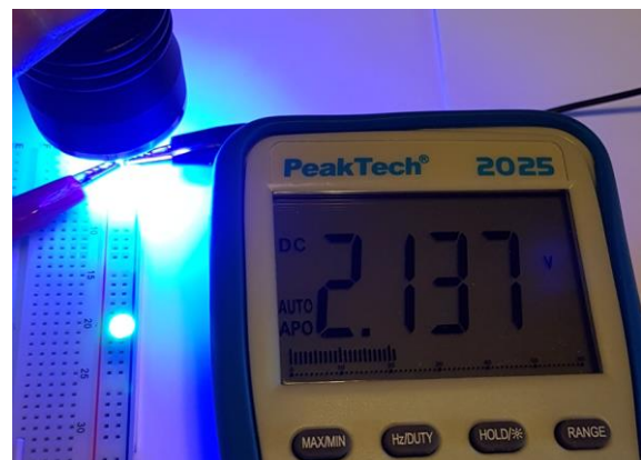
Fig.1: Students expose a blue LED to the light of a pocket lamp. The LED transforms the energy of the light into electric energy. With it, the connected green LED at pin 20 begins to shine. Moreover, the students attach two crocodile clips to the pins of the blue LED and to a Voltmeter. So they find out that the LED generates 2.137 V.
